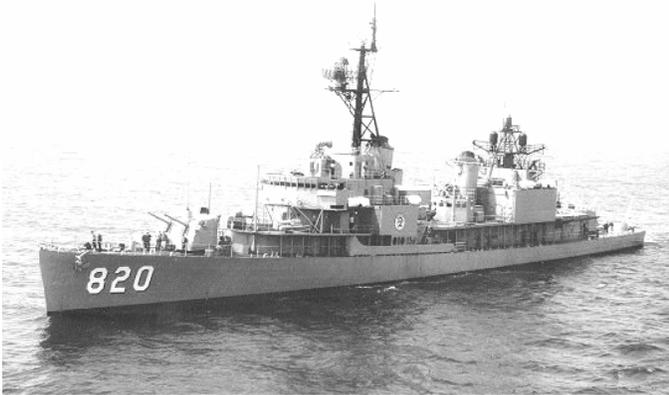
At a keel length of 390½ feet and weighing in at 3460 tons fully loaded the **RICH** was destined to be among the last of the steam turbine powered post World War II destroyers. Her conventional weapons also would be a thing of the past.
